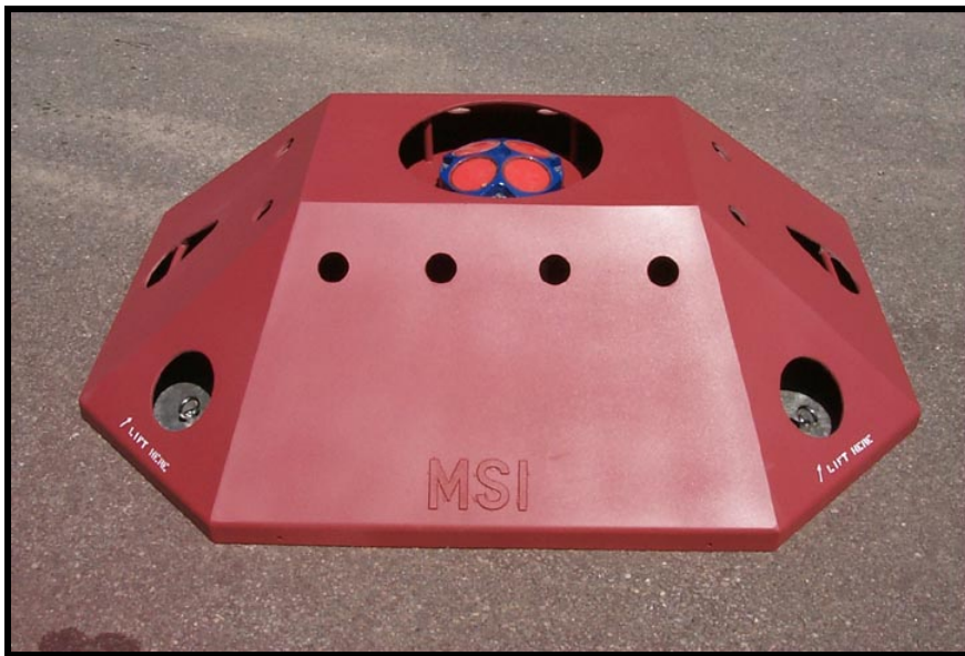
Figure 3-14. ADCP fitted in trawl-resistant bottom mount.
