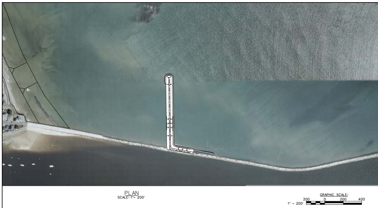
Figure 8-9. Alternative 6 plan form layout – with North Jetty reinforcement
