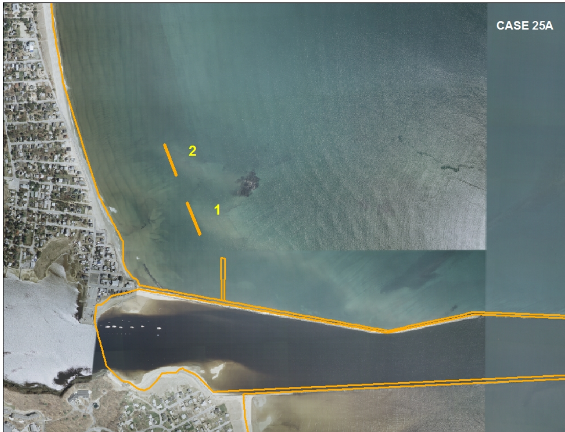
Figure 6-2. Alternative 25A: Segmented breakwater and spur jetty configuration 4 (modified).
