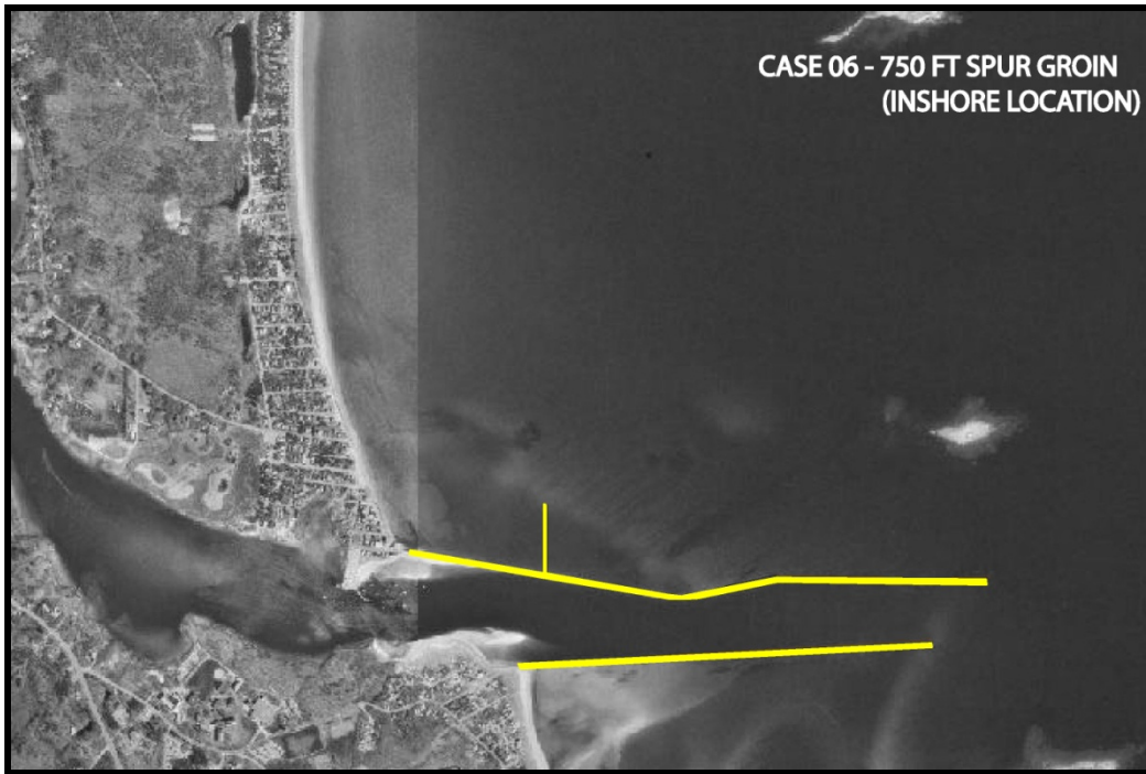
Figure 6-1. Alternative 6: Inshore placement of 750-foot spur jetty.
