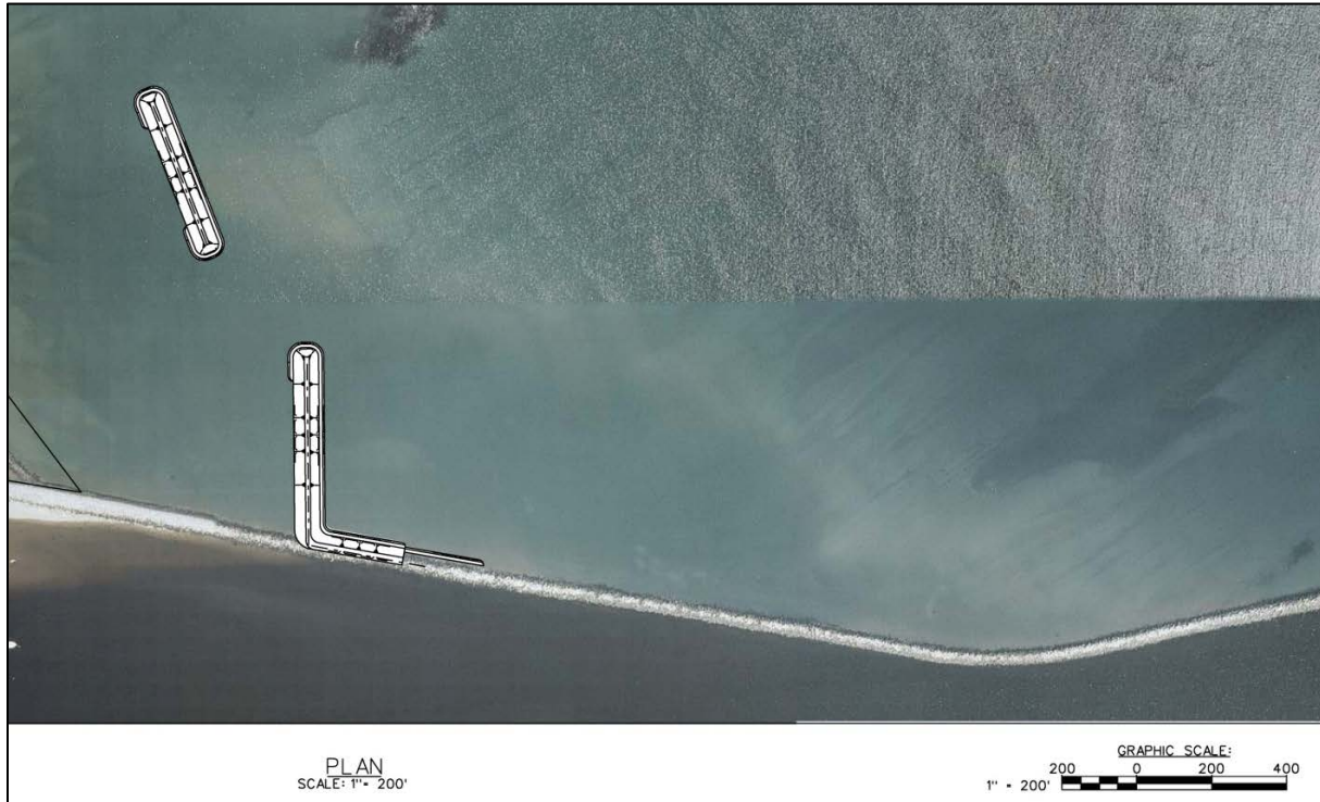
Figure 8-10. Alternative 25A spur groin plan form layout – with North Jetty reinforcement.
