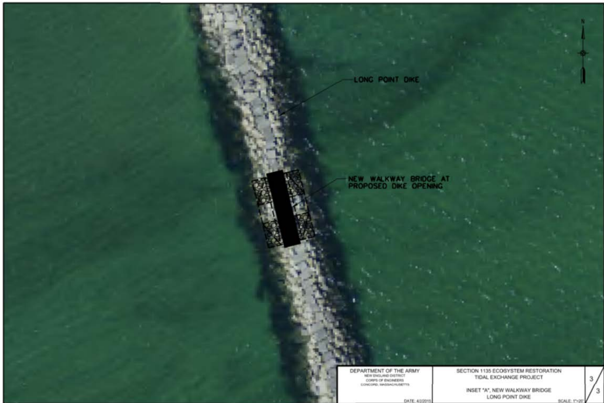
Figure 3 – Proposed Project Modification (single breach in dike)
