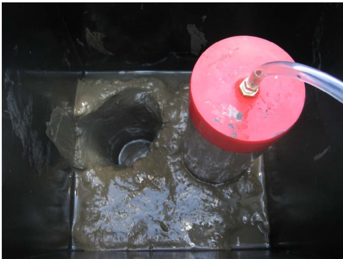
Figure 2-3. Box core subsampling with vacuum tube attached to core cap
