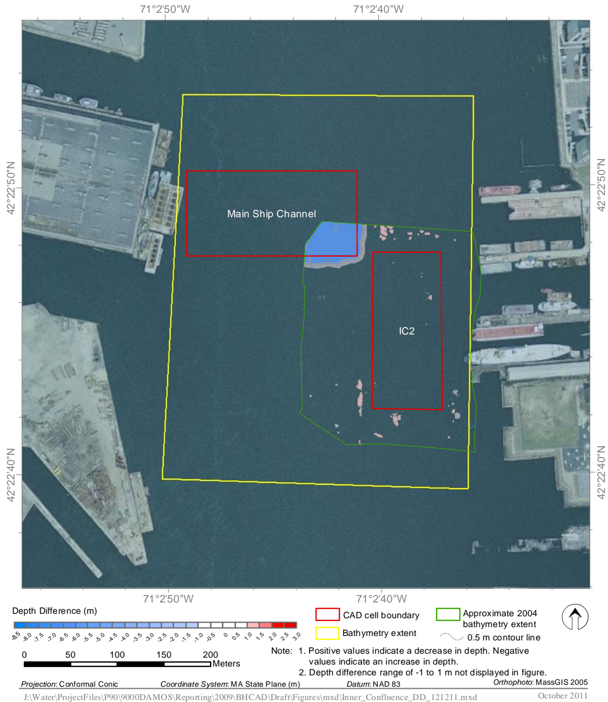
Figure 3-6. Main Ship Channel depth difference map, 2004–2009
